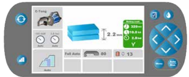
Choose between 4 welding modes, including fully automatic
